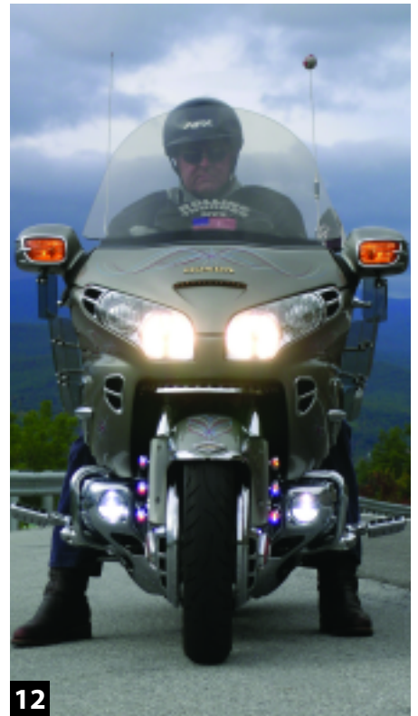
11 If the LEDs are aimed too high, you'll blind oncoming vehicles. With the bike on level ground, aimed at a wall about 16' away, measure the distance from the ground to the center of one of the fog lamps. Make a mark on the wall to that measurement. Tighten the adjuster screws on each fog lamp until they lower to that level.
