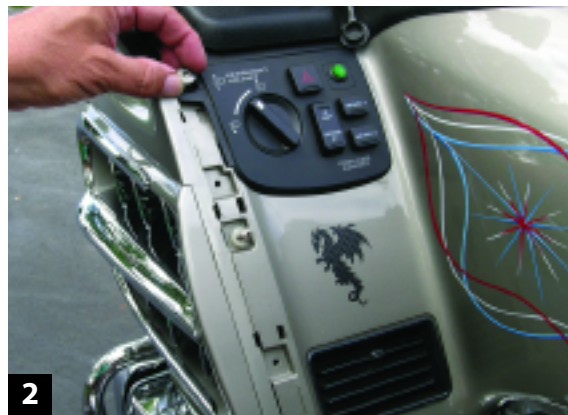
For the Air Wings with lowers, first remove the stock trim molding and two screws.
