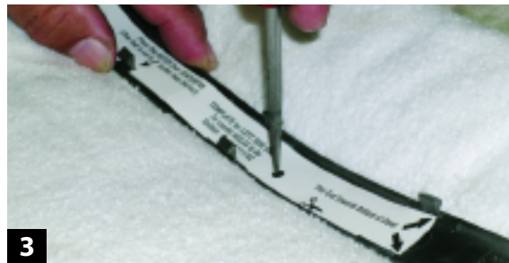
Cut out the supplied template and fit it to the inside of the molding. Then punch out the centers of the two circles to locate the screw mount points.
