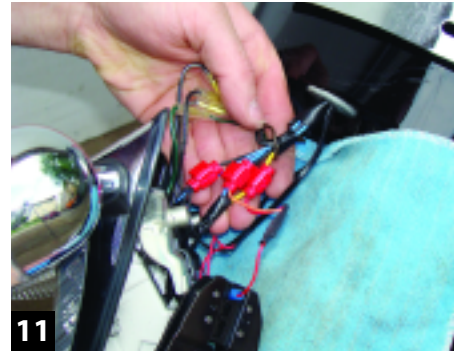
11 Tap into the stock signal and brake wires with scotchlocks.
