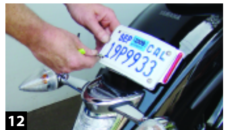
12 Once the lights were tested, I bolt the taillamp back in place and attach the license plate right-side bolts. Bend the plate over the arch of the bracket and affix the left bolts.
