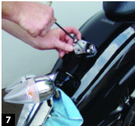
7 Start by removing the taillamp and resting it on a towel or cushion to protect the finish on the rear fender. The billet Rivco bracket bolts on with special drilled hollow bolts.
