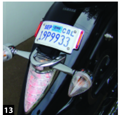
13 The LEDs provide extra running-light and brake-light visibility out back. The laydown plate hugs the rear fender line now. RB
