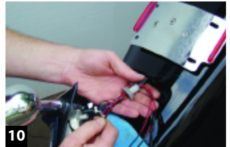
10 From inside the fender, feed the LED wires through the stock fender grommet toward the back of the taillamp. There's plenty of room in the grommet, but it's a snug fit.
