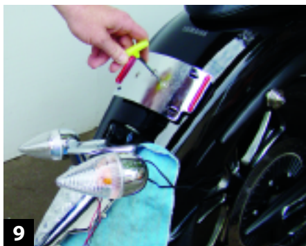
9 Feed the LED wires through the hollow bolts and attach the bracket. Be careful not to pinch the wires.
