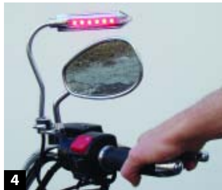
4 Once all the connections are made, the front and back LEDs shine yellow on turn signaling, and the back has red LEDs that light when the brakes are applied. RB
