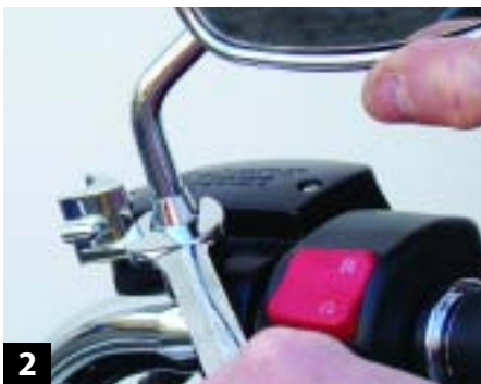
2 Remove the bike's mirrors, and sandwich the lower standoff bracket between the stock mirror and the handlebar control. Remember, some Yamahas have reverse-rotation mirror threads. Install the 2-BSEEN light to the standoff bracket, and tighten the two Allen head bolts.
