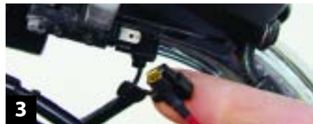
3 The handy little piggyback terminal tap is included with the kit and makes easy work of getting a brake light signal.
