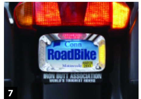
6 The result is a great-looking license plate frame that adds more visibility via a red LED running light that brightens when the brakes are applied...
