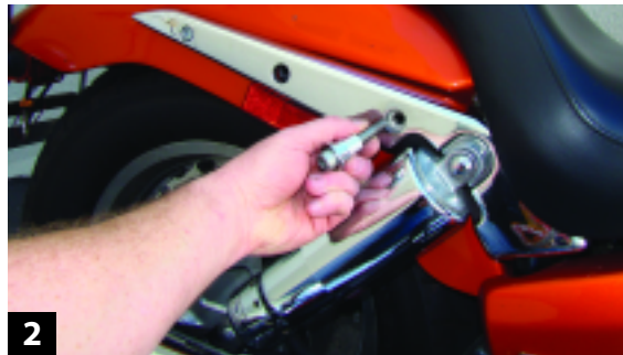
2 Find a location suitable for mounting the bolt lock T-washer. It'll accept up to a 3/8" or 10mm diameter bolt. Socket head cap screws work best. Dab thread-lock compound on the threads and reinsert the bolt mounted through the T-washer.
