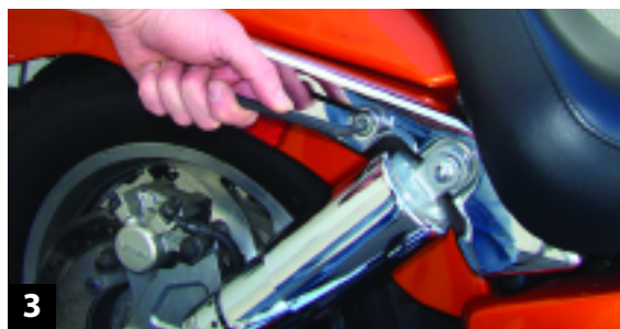
3 Loop the cable through your belongings, there's an eyelet at one end of the bolt lock cable. The bolt lock body will accept the flat end of the vinyl-coated cable.
