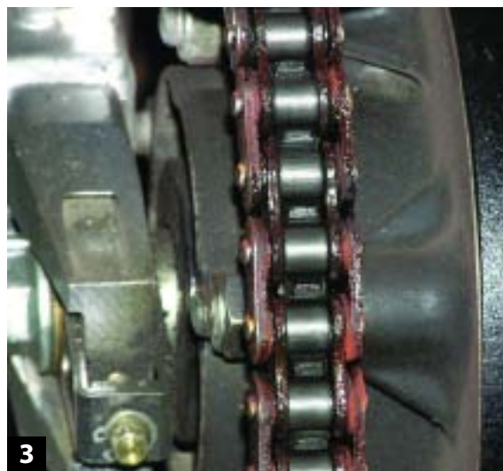
3 In case there was any doubt, this is what a bad chain looks like. This one is way past its prime.
