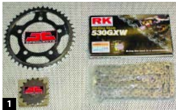
1 JT sprockets and RK chain make nice replacements for the war-torn factory parts.
