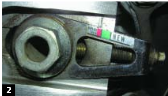
2 You can't argue with this gauge. Factory axle adjusters on some bikes have indicators to tell you when it's time for a new chain.
