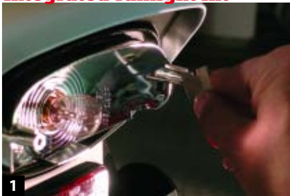
1 After removing the stock brake light lens, you need to cut off the two plastic ridges on each mounting stalk with a sharp blade.
