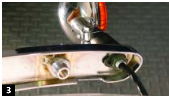
3 We had to remove the stock V Star's turn signals to accommodate the saddlebags. We removed the fender struts to access the signal stalk bolts.
