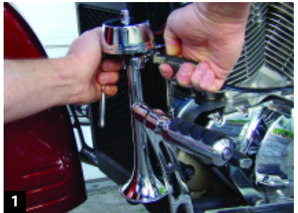
After checking for front-fender clearance, I mount the large horn to the left-frame downtube.
