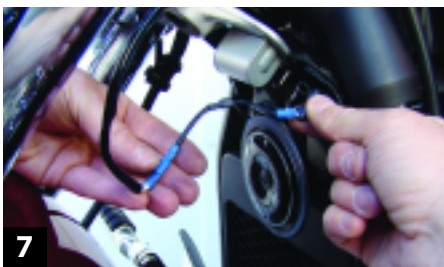
7 Disconnect the factory positive lead from the OEM horn and connect it to the Kuryakyn wire harness with the Y-lead. Wrap the wires and tuck them out of the way. The wimpy stock horn is still there, but you really hear the trumpets. RB
