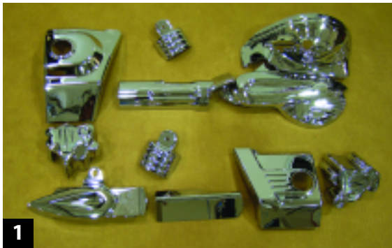
1 Küryakyn chassis chrome parts include driveshaft covers, frame trim, and shock absorber caps.
