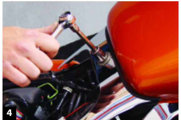
4 First, the seat is removed, and the tank trim attaches via the stock tank hold-down bolt.
