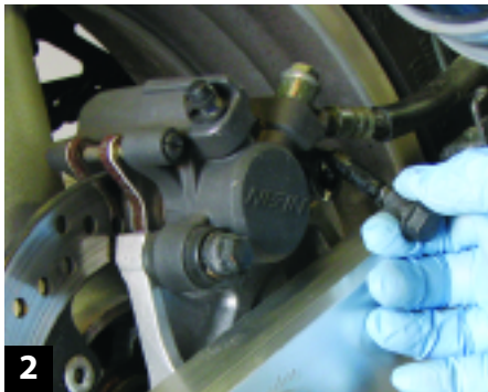
Starting with the rear brake, loosen the pad pin (the pin that holds the brake pads in the caliper), then remove the two bolts holding the caliper to the swingarm, before finally removing the pad pin and pads.
