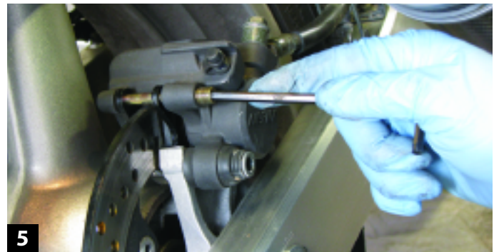
Tighten the bolts holding the caliper in place, and then tighten the pad pin bolt. I put a little anti-seize on each bolt to prevent corrosion and galling.
