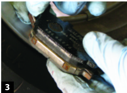
Check the new pads against the old ones, making sure they match up before installing.
