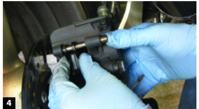
Compress the caliper piston, install the new pads and pin, and slide the caliper back on the disc.
