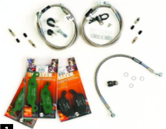
1 A fresh set of Galfer pads and stainless steel braided lines from Russell.
