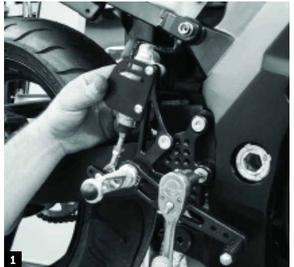
1 First, Chris attached the rear brake master cylinder to the right-side reseat, and then bolted the reseat onto the bike. Sweet!
