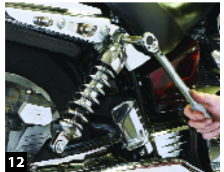
12 Using the frame jack, adjust the bike to the correct height so the new shocks can be installed.
