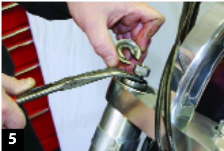
5 Twist the lock nut onto the damper rod, and slip the slotted retaining washer in between the lock nut and spring collar.
