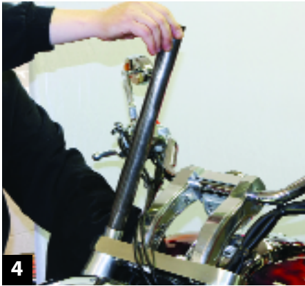
4 Reinstall the original spring collar next.
