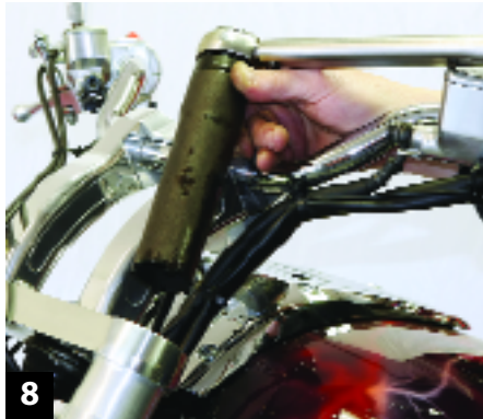
8 Tighten rebound rod assembly to factory specs using the Honda Special Tool.
