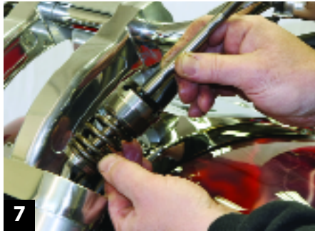
7 Now install the rebound rod assembly.
