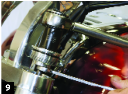
9 Thread on the fork cap lock nut, and tighten just enough to hold the cap. Repeat on the right leg.
