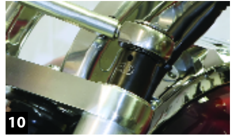
10 Next we raise the support jack and tighten the fork caps to factory specs. The fork is done.
