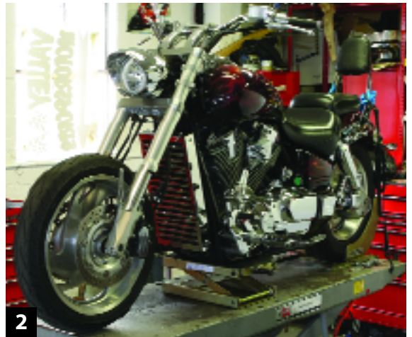
2 Support the front end with a frame jack, remove fork caps, and slowly lower the jack to remove the stock fork springs per Honda's service manual. The two legs are different inside, and the left one requires a Honda Special Tool (available from your local Honda dealer) to remove the damping rod assembly.
