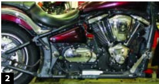
2 First, the stock exhaust system, right-side floorboard, and stock muffler support bracket are removed. (Note: the rear brake line should be disconnected first in order to remove the muffler support bracket.)
