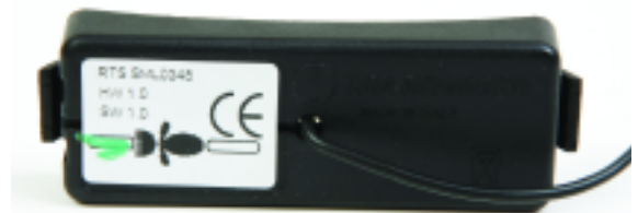
Sensors are particular to front and rear wheel (they're marked; front shown).
