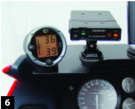
5 Mount the dash gauge in clear view of the rider. It's operated by a self-contained battery.
