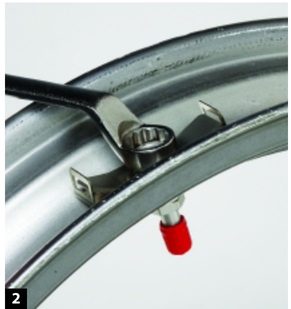
Demount the tires and install the new ZADI valve stems on the wheels. This metal bracket will hold the sensor.
