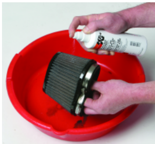
Apply the cleaning agent to the dirty filter, let it soak, and then rinse from the inside out using gentle tap water pressure.
