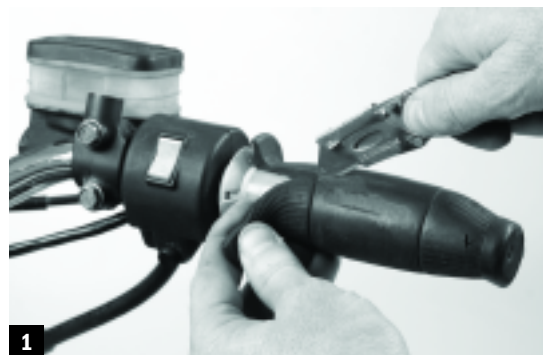
1 You can use a sharp knife to cut off the old grips. Or try blowing compressed air into the ends while working them off.
