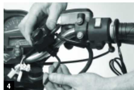
4 Install the handlebar mounting bracket in a convenient location. The thermostat attaches with double-sided tape.
