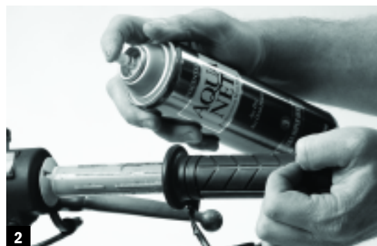
2 Hairspray makes a good adhesive for the new grips. It stays slick for a few seconds, letting you slide the grips in place before it becomes tacky.
