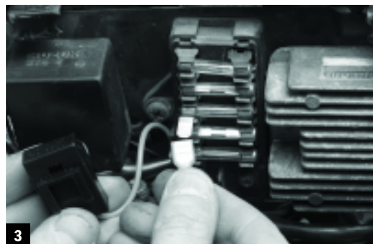
3 Remove (or lift) the gas tank to run wires to the fuse block. Attach the red wire to a live terminal when the ignition is on; black goes to the chassis ground.
