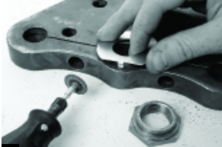
8 The original front wheel had no center bearing spacer. Kenny Buchanan made us promise we'd tool one up before we reassembled his beautiful wheel. Another wrong set right.
