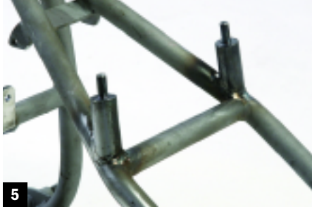
4 Check out the new brake stay tab on the frame. The old one is shown alongside it. It made us cringe to think someone would use a tack-welded carriage nut to hold the only brake on the bike.
