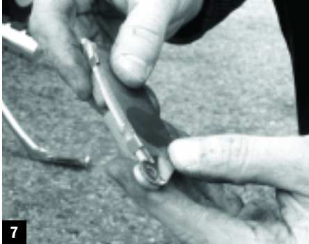
7 Steve removed the clip from the original pad, cleaned it with brake cleaner, and snapped it onto the new pad.
