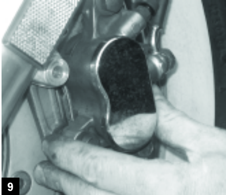
9 Getting the caliper back in position wasn't the struggle I'd expected, because Steve had pushed the pistons apart enough (step 4).
