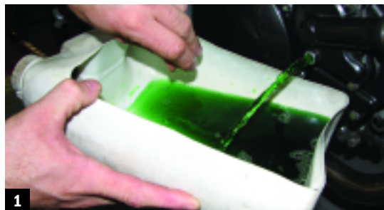
1 Drain the system entirely, or as much as possible. Don't forget that some bikes have multiple drain points.
