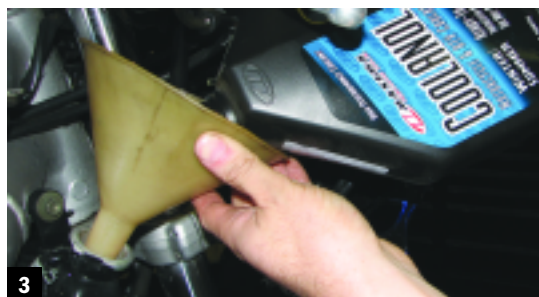
3 The highest point in the system is usually the radiator.
