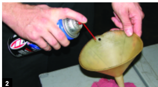
2 Anytime you're using a funnel to pour fluids into a system, it's a good idea to clean it first. We used spray brake cleaner.
