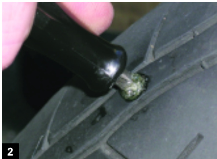
2 He applied a generous amount of cement to the plug tool, stuck the tool in the hole, and rotated it back and forth to distribute the cement evenly and ream the hole. You'll be pushing on the tire forcefully, so make sure the bike's in gear and hold onto the rim.
