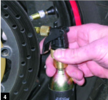
4 After letting the cement dry for 15 minutes, Steve pieced together the CO2 cartridge assembly and threaded the adapter hose onto the tire valve stem. Holding the cartridge vertically while pressing the trigger, it took only about five seconds to empty it. But be careful: The cartridge freezes when you do this, and it can hurt to hold it.
