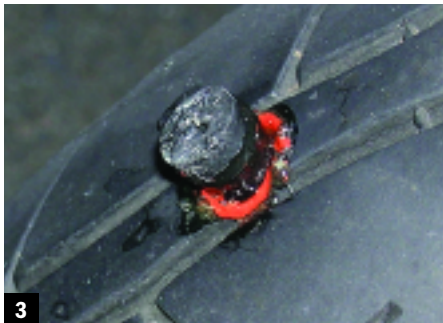
3 Trying not to handle the sticky part, Steve placed the plug on the tip of the tool. He coated the plug with more cement and pushed it as far as possible into the hole. He then trimmed the plug with a sharp blade, leaving about 1/8" of rubber outside the tread. (It'll get flattened a bit once you get rolling.)
