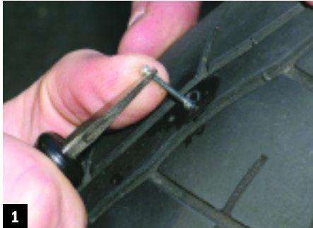
1 After determining that a nail was the source of the leak, Steve pulled it out.
