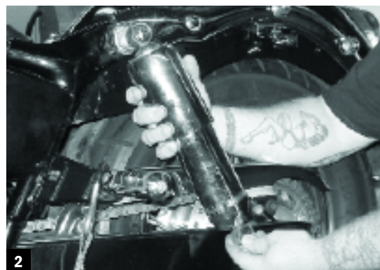
2 My 440s were an inch shorter than stock, so we had to pull off both stock shocks before installing the new ones.
