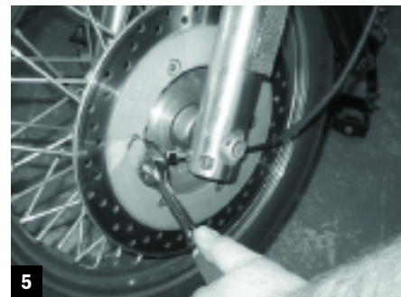
5 Moving on to the fork springs, he removed the brake calliper, loosened the axle nuts, removed the four pinch bolts...
