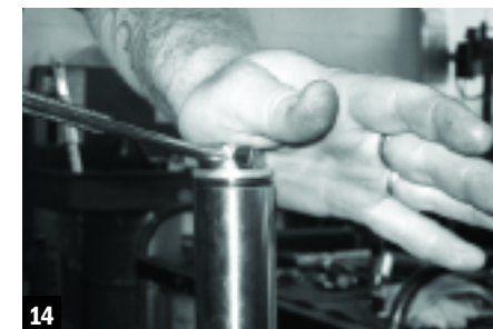
14 Paul pushed down while tightening the fork cap. You should be careful to put it on straight from the first turn, because it can very easily get cross-threaded.
