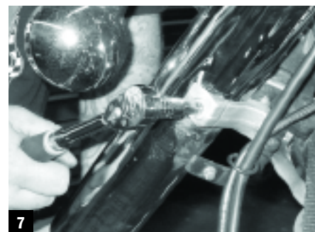
7 Next, Paul loosened the pinch bolts that hold the forks to the triple trees.
