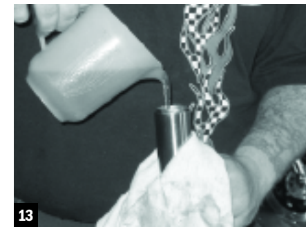
13 Referring to the owner's manual, he measured 16 ounces of 20-weight fork oil and carefully poured it into the fork tube. He did the same with the other fork.
