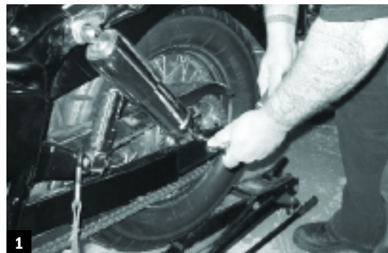
1 Paul stabilized the rear tire with a jack, removed the two bolts holding the stock shock, and then removed the shock. If your new shocks are the same size as the stockers, you can install one now.
