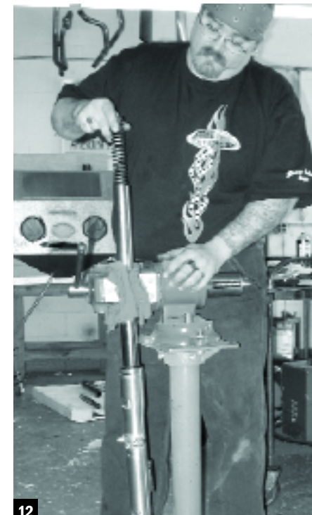
12 With one fork held stable on the bench press, Paul dropped in the Progressive spring, followed by the stock washer, then the 5" spacer.
