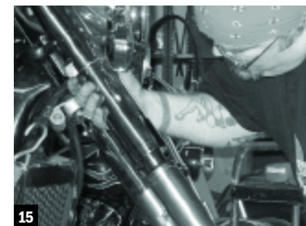
15 After spraying a bit of Teflon lube on the fork tube, Paul twisted it back into position and tightened the pinch bolts.
