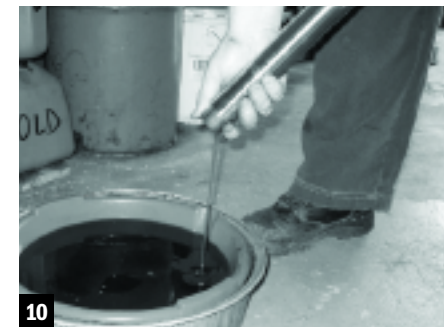
10 Paul drained the fork oil into a vat of old oil (to be recycled later).
