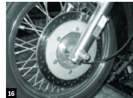
16 Finally, he bolted the fender back on, sprayed some anti-seize on the axle, and remounted the wheel and brake assembly. By the way, if you're thinking of replacing your brake pads, this would be a great time to do it. RB
