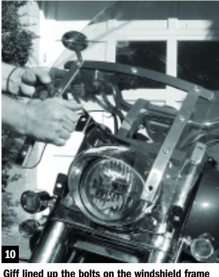
9 With the supplied washers and acorn nuts, he installed the upper and lower windshield bracket to the headlight surround.
