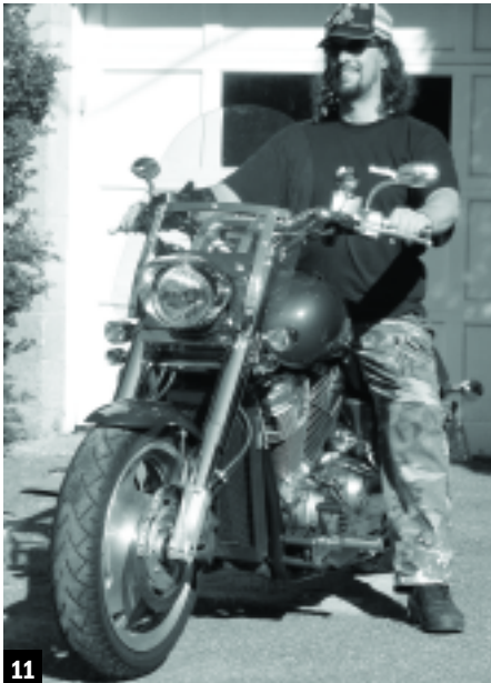
11 Finished! Giff's happy with his slick new windshield. And the bolt-on mount kit makes it simple to remove or replace. RB
