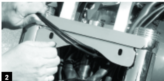
First, Giff installed (fingertight) the upper mounting base to the upper triple tree with hex head screws, making sure the cables were in the center section of the upper bracket.
