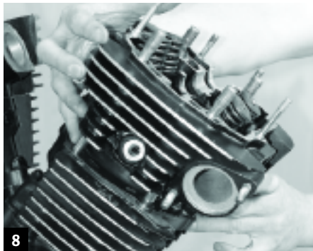
8 Rich then slid the heads onto the motor.
