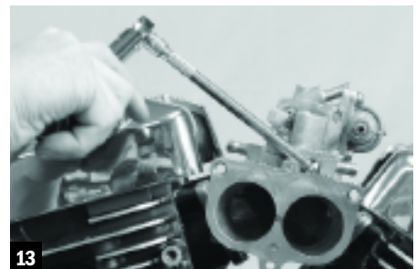
13 Finally, Rich bolted the throttle body to the intake manifold...
