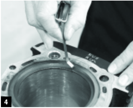
4 First, Rich checked the ring end gap by putting each ring in a cylinder and measuring the gap with a feeler gauge, going by the specs in the kit instructions. (If the numbers don't match, the rings need to be ground.) Then, before installing the pistons, he put a clean rag inside each cylinder bore, to prevent small parts from falling into the motor.
