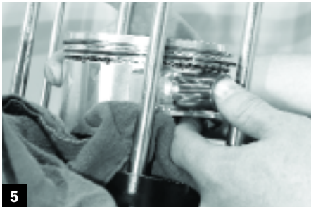
5 Rich put the rings on each piston, staggering the end gaps according to the instructions. He snapped in a circlip, put assembly lube on the wrist pin and pushed it through the piston and connecting rod, and then snapped the second circlip in place. The pistons are oriented according to the size of the valve pockets — the smaller pockets (for the exhaust valves) face forward in the front cylinder and rearward in the rear one.
