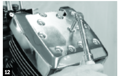
12 He put the brass lifter oil filters back in the rocker box and filled the oil reservoirs. Then he installed a new valve cover gasket and torqued all the bolts to spec. Moving on to the rear cylinder, he repeated steps 9 through 12 to complete the valvetrain assembly.
