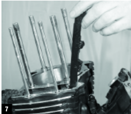
7 Next up were the cam chain guides (marked "front" and "rear"), head gasket, and locating dowels.
