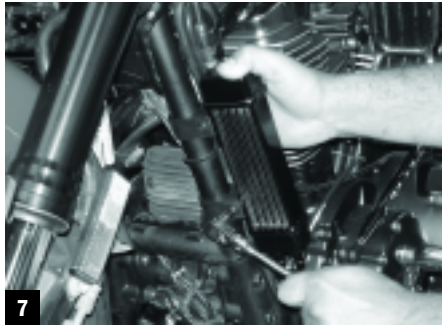
7 The oil cooler gets mounted to the left-side frame downtube. Two different size clamps are provided with the kit; the Warrior uses the larger of the two.
