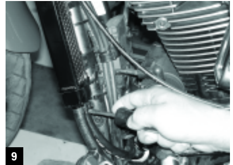
9 Slip the other ends of the lines onto the oil cooler barbs and tighten the four hose clamps.
