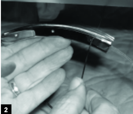
1 First, Pete added an extra chrome adhesive strip to the inside of the light bar to give it a tighter fit.
