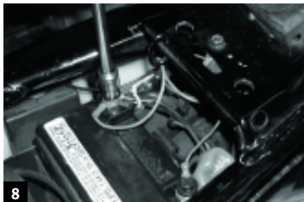
7 Pete gathered the hot (red) wires in one bundle and the ground (black) wires in another, near the area where the switch would go. He soldered one of the switch wires to the bundle of red wires and the other switch wire to the 3-amp fuse holder. The switch was then mounted near the fuel petcock valve.
