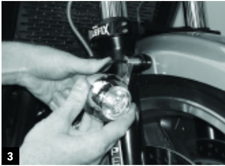
3 Bolt the entire assembly to the bike's front fender. A longer stainless steel bolt is provided, and a drop of blue Loctite will ensure that it won't vibrate loose.
