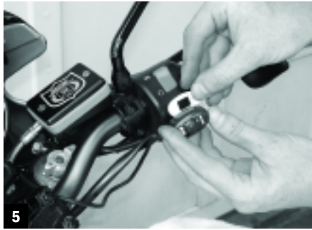
5 The waterproof switch mounts up near the grip with double-sided tape. A green LED shows power, and a red LED indicates when the lights are on. Be sure to allow for the full range of handlebar travel when you route this wire lead.
