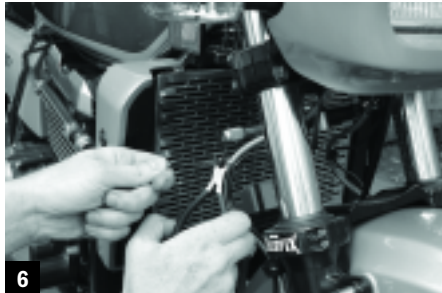
6 Tuck all wires away, leaving plenty of slack for suspension travel. I ran them along the brake hose and held them in place with zip-ties.
