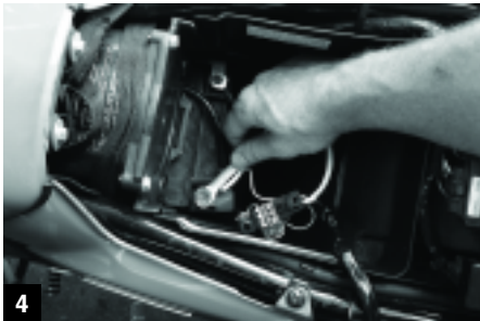
4 The pre-made wire harness attaches directly to the battery. There's an inline fuse and relay built into the harness. Run the wires under the tank to the front lamp's pigtails.
