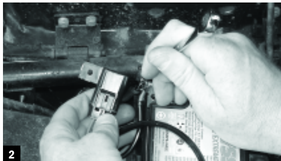
Simple wiring. The red attached directly to the positive battery terminal, and the black to a chassis ground bolt.
