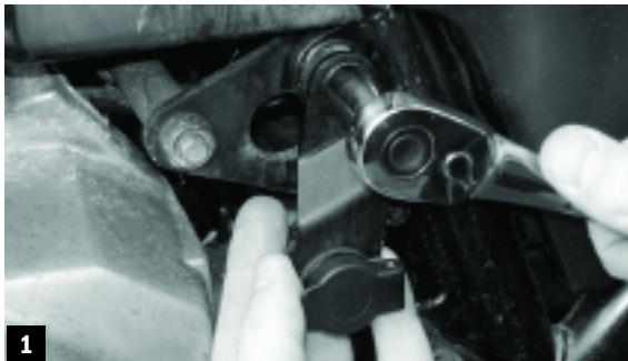
After deciding to mount the outlet on my bike's left motor-mount bolt, installation was easy.
