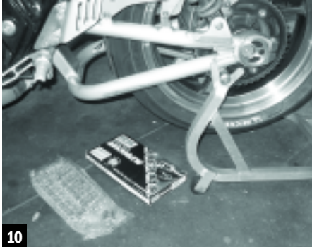
10 Here's my new chain, ready for fitment on the reinstalled wheel. RK ships its chains pre-lubed.
