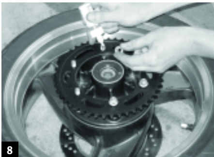
8 It's not a bad idea to use some liquid thread lock on the nuts. (This bike had red Loctite from the factory.)
