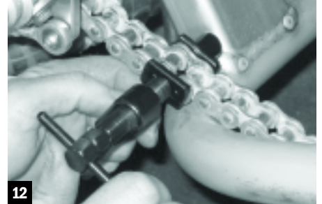
12 Use care when you're pressing the outer plate onto the chain. Press too far, and you could cause it to bind. I did this procedure in several steps, checking periodically as I went.
