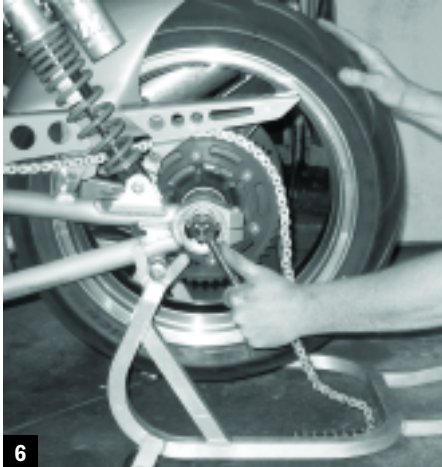
6 Remove the rear wheel for gear replacement. Make a note of any markings or offset on the OE sprocket.
