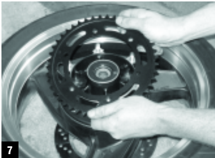
6 Remove the rear wheel for gear replacement. Make a note of any markings or offset on the OE sprocket.
