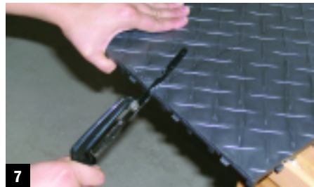
7 ...and cut the tile with a small saw. I later used a circular saw, which was much quicker and easier.
