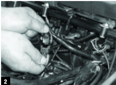
2 The male ends on the PCIII harness snap into the Triumph harness, and the female ends clip onto the injectors. Start on the far left of the engine with the orange-wired PCIII connector.
