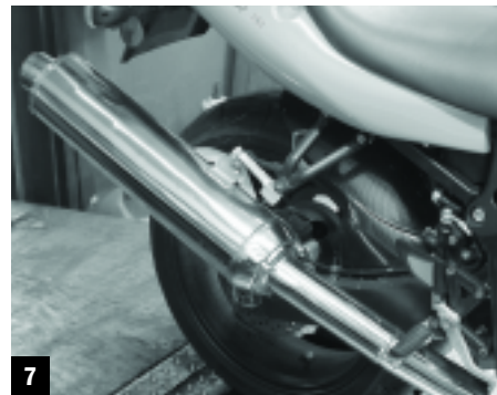
7 The stock Triumph muffler is much larger and heavier than the Two Brothers unit.
