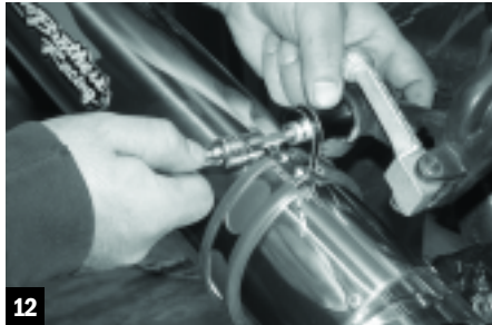
12 The exhaust clamp is then bolted to the stock footpeg bracket with the provided spacer. Be sure to remove the plastic protective sheet on this clamp before you start the bike.
