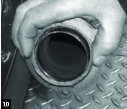
10 Then slip the original gasket back into place on the shortened flange.
