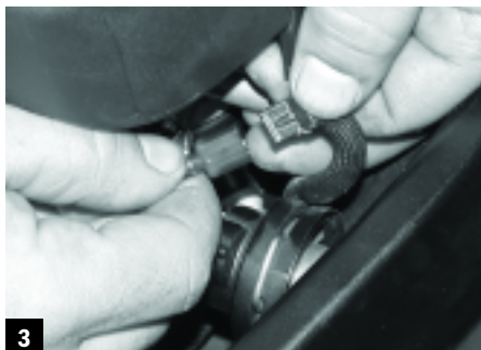
3 Tap the gray wire from the PCIII to the yellow wire on the throttle-position sensor with the supplied Scotchlok connector.
