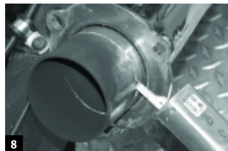
8 We started by modifying the head pipe with an air-powered saber saw. We trimmed the rear flange down to .5", first removing the right rear footpeg bracket to make room to work.
