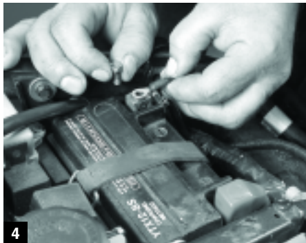
4 Next, attach the ground cable directly to the negative battery post, and attach the PCIII to the inner rear fender with Velcro.
