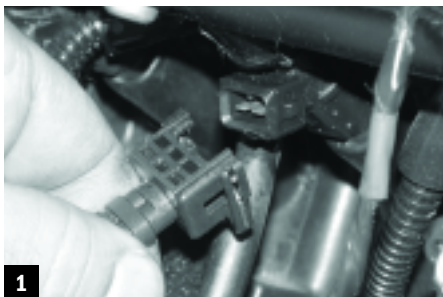
1 First, remove the seat and tank, and disconnect the factory fuel injector wire harness by squeezing the spring clip on each connector. You don't need to remove the clips.
