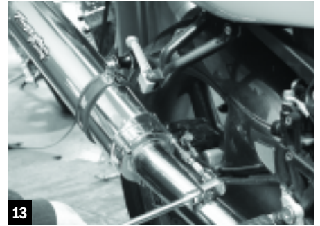
13 Finally, evenly tighten the three flange bolts at the end of the can, and clean the can thoroughly with rubbing alcohol – you don't want to leave greasy fingerprints permanently etched into the finish.
