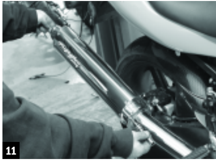
11 Now you can slip on the Two Brothers can. It should be held in place loosely with the original three bolts. After that, we replaced and tightened the rear footpeg bolts.
