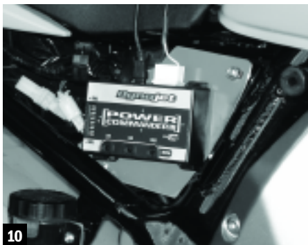
10 Dynojet suggests putting the controller in the tool tray, but I mounted it inside the right side panel with the provided Velcro.
