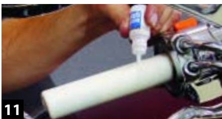
11 Grip cement is applied to keep the grips in place once installed. Work quickly to align the ISO grips.
