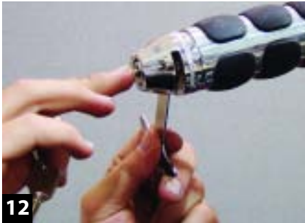
12 The KewlMetal bar ends attach to the ISO grips with supplied screws. They incorporate a keyed lock pin so you can secure your helmet.
