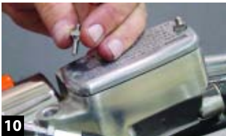
10 Ingenious ministuds replace the stock Phillips head screws on the brake master cylinder. They hold the chrome master cover securely in place.
