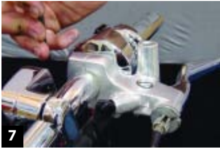
7 ...tighten the clutch perch in place.
