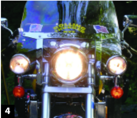
4 ... to bright. To turn the modulator off, just switch the headlight to the regular (not high) beam setting.
