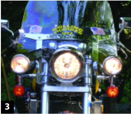
3 We reinstalled everything and tested our unit. When the daylight is bright enough, the modulator flashes from dim ...
