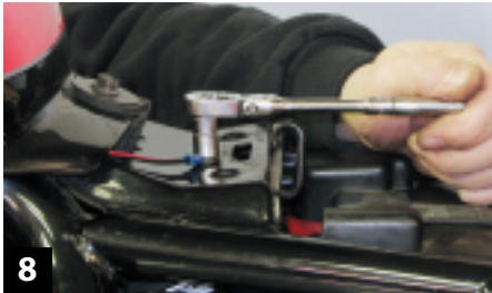
8 Using the supplied wire harness, run it through the rear of the headlight basket, crimp the ground lug onto the wire and secure it to a chassis ground.
