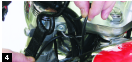
4 Route the speaker wires through the handlebar looms.
