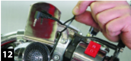
12 Run the audio cable with jack up the right handlebar and secure it to the MP3 mount.
