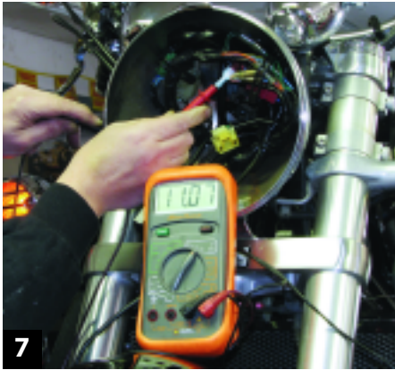
7 Remove the headlight unit from the basket, then locate a power wire that has power only when the ignition switch is turned on.
