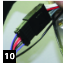
10 Plug the speaker wire connector into the amplifier connector.
