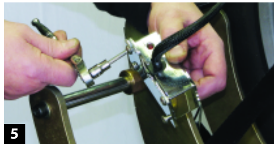
5 Mount the amplifier to the amp mounting bracket.
