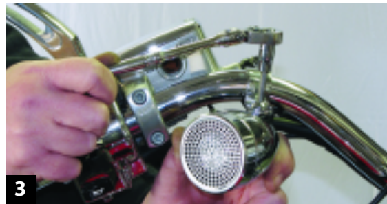
3 Mount the speakers on handlebars using the included brackets.
