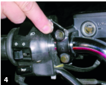
4 ...then mount the bracket to the brake master cylinder.
