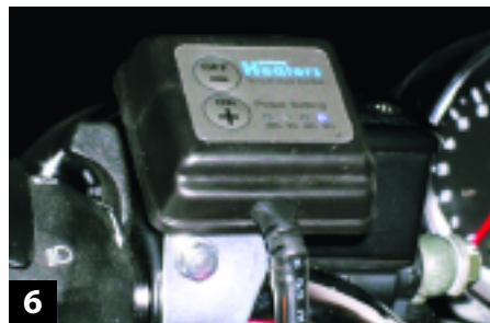
6 To test the HotGrips, I ran the motorcycle in order to allow enough voltage through the temperature controller. Make sure that all wires are neatly tucked out of the way, don't interfere with any controls, and have enough slack for turning the handlebars and twisting the throttle.
