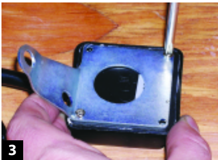
3 The temperature controller can be mounted to a fairing or other flat surface with the included double-sided adhesive, or you can use the provided metal bracket. First use the screws to fix the controller to the bracket...
