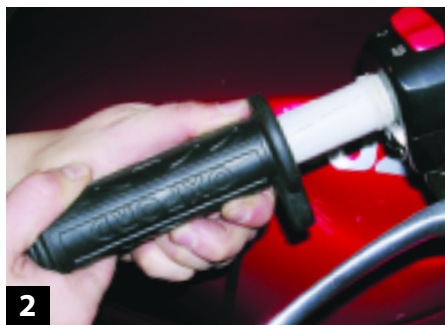
2 Remove the stock bar-end weights and grips. Test the Oxford grips to make sure they fit, then use some grip glue before permanently installing them on the handlebar. It was a tight fit, but I was able to twist them into place with a bit of effort.
