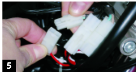
5 After connecting the negative and positive ring terminals to the bike's battery, I routed and zip-tied the wires from the battery along the frame to the steering stem. The two grip wires and the battery lead all click into the controller via multipin block connectors.
