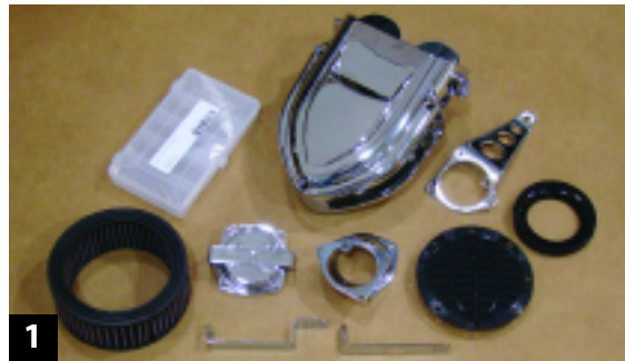
1 All the parts, fresh out of the box: the jet kit and genuine K&N filter are included.
