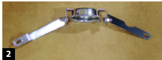
2 Preassemble the replacement chrome carb cap, but don't tighten the bolts at this time.
