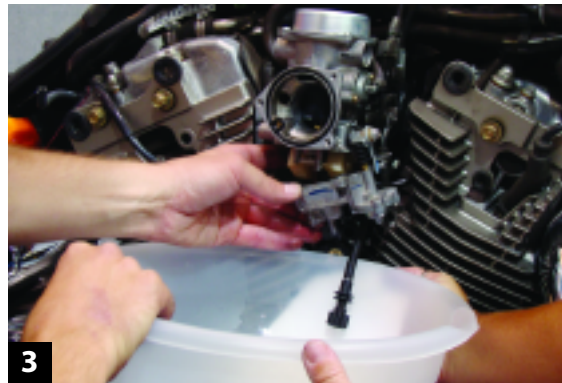
3 Remove the seat, prop up the tank, and then remove the stock air cleaner and spark plug covers. Luckily the entire rejet can be done without removing the carb from the engine. Drain the fuel bowl, and remove it to gain access to the jets.
