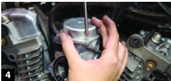
4 Remove the four screws holding the stock carb cap on.
